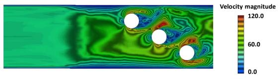
Figure 1. Cross-sectional view of the flow past three cylinders from 3D computation. The velocity magnitude is in m/s, and the cylinder diameter is 2 cm.
